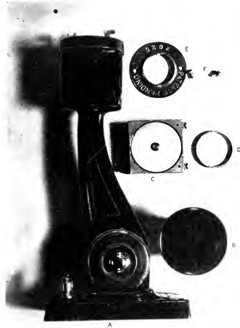
FIG. 48.—FAHNESTOCK TRANSMITTER DISASSEMBLED.
